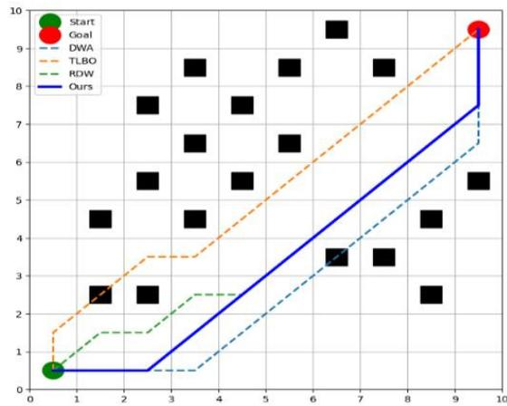
Figure 2. 10x10 Grid World Environment with Navigation Paths.
