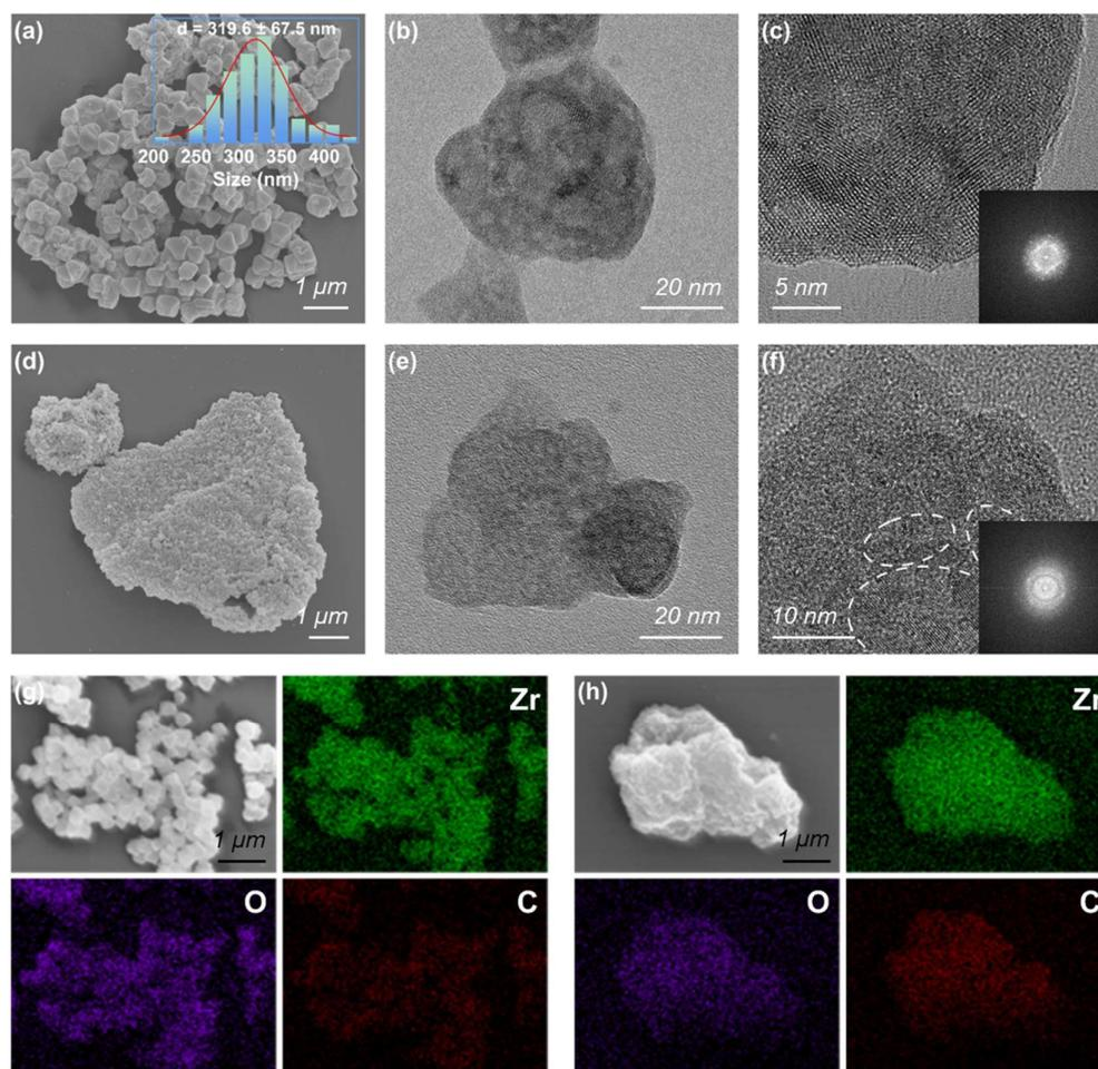
**Figure 2** The SEM, TEM, and EDS images of powder and monolithic MOF-801. The morphology and the Fast Fourier transformation (FFT) spots for (a, b, c) the powder MOF-801 and (d, e, f) the monolithic MOF-801. The elemental mapping of Zr, O, and C of the regions for (g) the powder MOF-801 and (h) the monolithic MOF-801.
