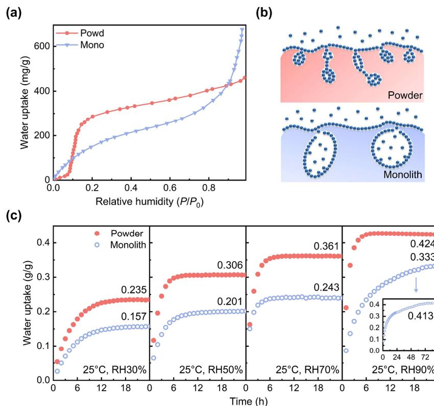
**Figure 4** The water uptake of powder and monolithic MOF-801. (a) The water vapor adsorption isotherms of powder and monolithic MOF-801. (b) The schematic of water adsorption mechanisms in powder and monolithic MOF-801. (c) The on-site water uptake tests of powder and monolithic MOF-801 at 25 °C and RHs of 30%, 50%, 70%, and 90%.
