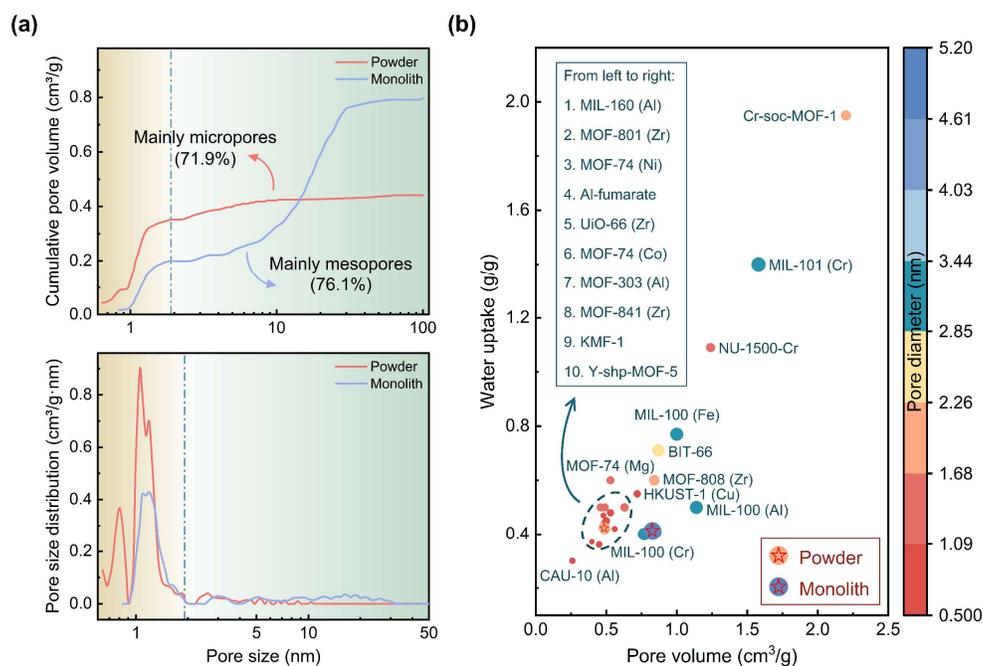
**Figure 3** The water uptake capacity and pore size distribution of powder and monolithic MOF-801. (a) The Non-Local Density Functional Theory (NLDFT) cumulative pore volume and pore size distribution of powder and monolithic MOF-801 as a function of pore size. (b)
