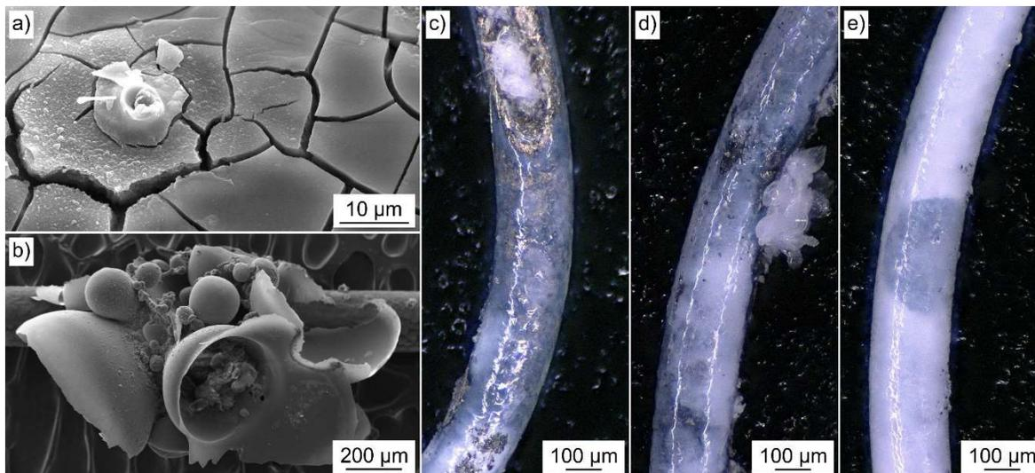
Fig. 4: Corrosion of ultra-pure Mg wire in  $\alpha$ MEM+FBS. a) Redeposition-stimulated nucleation of fine corrosion products after 2 hours near a corrosion site, b) open and closed corrosion products formed on H<sub>2</sub> bubble cluster after 24 h, c-e) 3D light microscopy images of the wire after 1 h, 24 h and 15 days.
