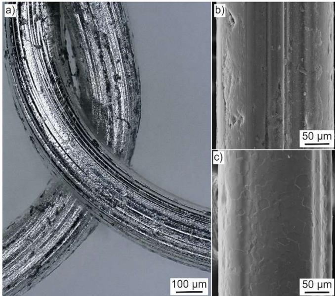
Fig. 1: a) 3D light microscope image of as-extruded 250 µm Mg-0.4Zn wire b) SEM comparison of the ultra-pure Mg cleaned in acetone and c) cleaned via Nital pickling.
