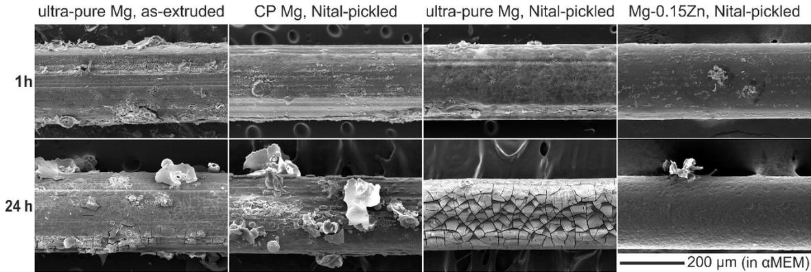
Fig. 3: Typical SEM micrographs of the degradation morphology of uncoated thin Mg and Mg-Zn wires in  $\alpha\text{MEM}+\text{FBS}$  after 1 and 24 hours.
