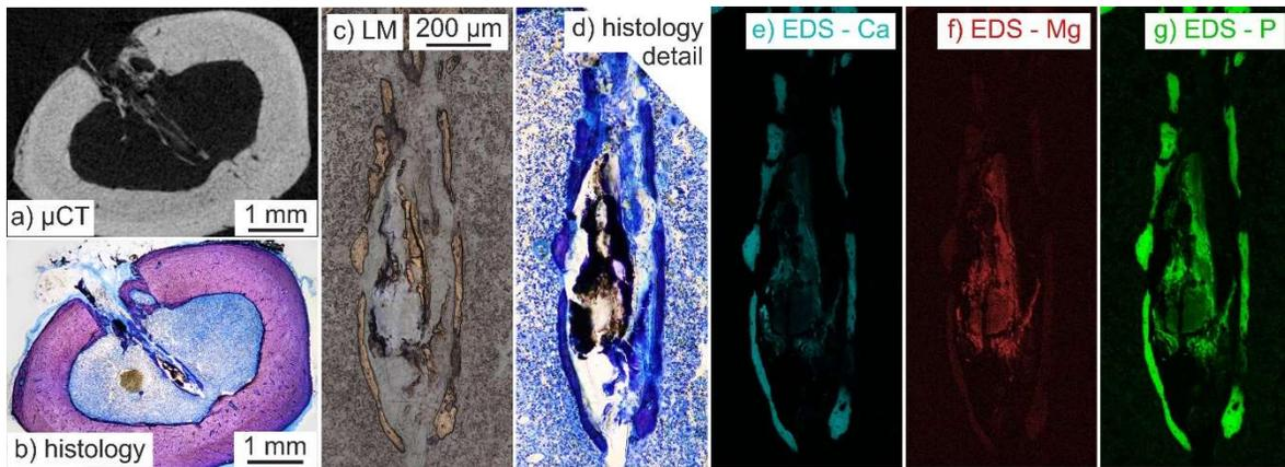
Fig. 9 Distal defect with remnants of degraded polymer-coated Mg-0.4Zn wire and a convex shape of a bone tissue envelope a)  $\mu\text{CT}$  cut, b) histological slide, c) LM image of Mg-induced osteogenesis, d) histological detail, e-g) SEM-EDS maps.
