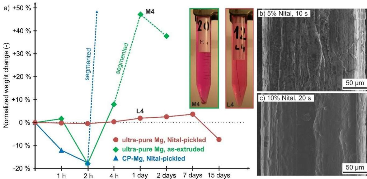
Fig. 8 a) Graph depicting normalized weight change of a dried uncoated Mg wire with respect to material purity and surface condition in  $\alpha$ MEM, b) and c) SEM image of Mg-0.4Zn wire surface after 10 s in 5% Nital and 20 s in 10% Nital, respectively.
