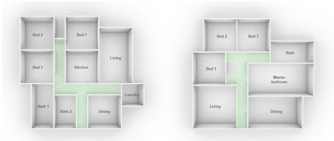
Figure 9. The space allocation and circulation pattern of two houses generated by the proposed generative design framework (and rendered in Rhino 7).
