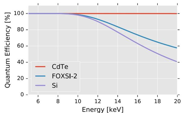
Fig. 5. The quantum efficiency of the 0.5 mm thick *FOXSI-2* detectors. Silicon (Si) efficiency falls to  $\sim 40\%$  at 20 keV while the CdTe efficiency remains almost unity throughout the *FOXSI* energy range. The average quantum efficiency for *FOXSI-2*, which contains 2 CdTe and 5 Si detectors, is also plotted.
