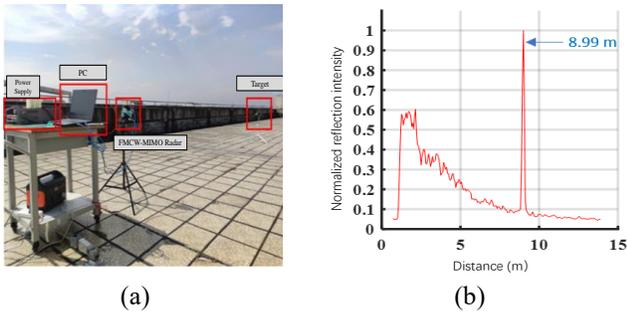
Fig.11. Range resolution analysis with (a) the experiment scenario deployment and (b) the measured range profile of the target.
