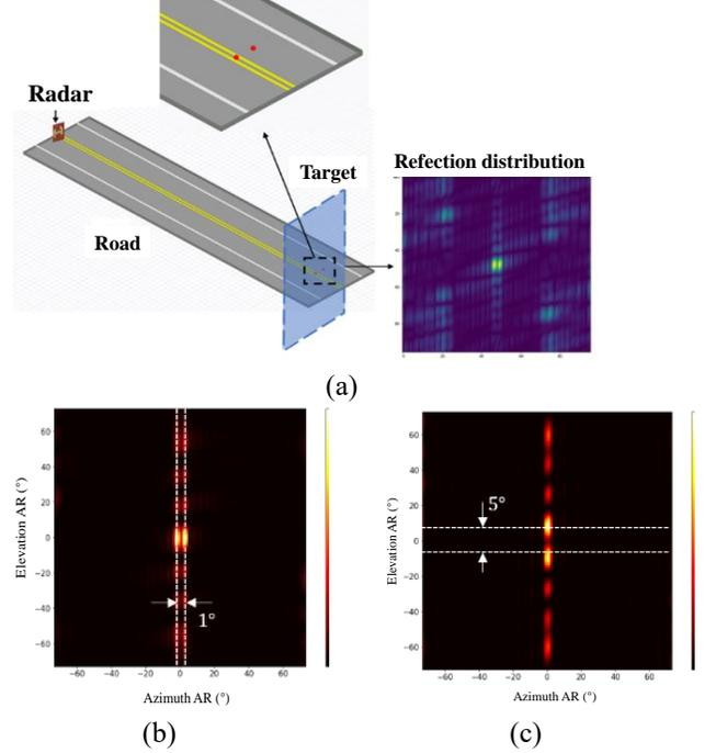
Fig.10. Simulation analysis of the designed MIMO array with (a) SBR tracing geometry and reflection distributions of two objects in (b) horizontal direction and (c) vertical direction.
