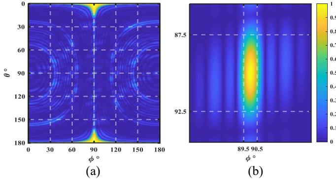
Fig. 5. The resolution analysis of the designed array with (a) ambiguity function map and (b) detail of the ambiguity function map.
