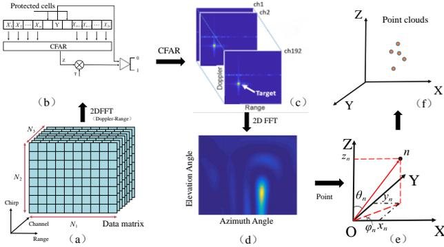
Fig. 1. The mmWave radar point cloud imagery diagram
