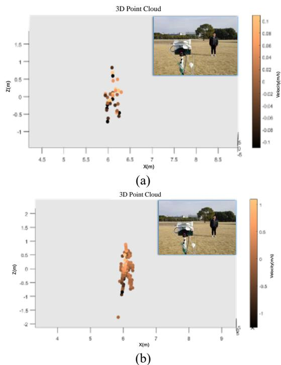
Fig. 16. The pedestrian imagery experiment (a) the original method of TI AWR2243 and (b) the proposed method.
