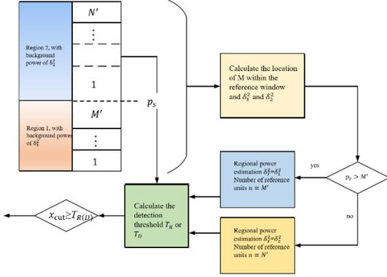
Fig. 7. The diagram of the proposed dynamic CFAR.
