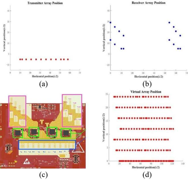
Fig. 4. The designed ladder shape array with, (a) the transmitter antenna array, (b) the receiver antenna array, (c) the physical MIMO array and (d) the final virtual array.
