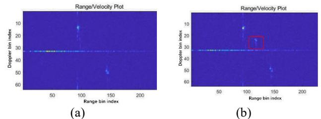
Fig.14. Weak target detection using (a) the original manufacturer patch antenna of TI AWR2243 and (b) the optimized antenna designed in this paper.
