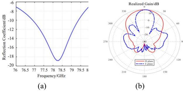
Fig. 3. The performance of the antenna design, (a) reflection coefficient of simulation, and (b) realized gain.
