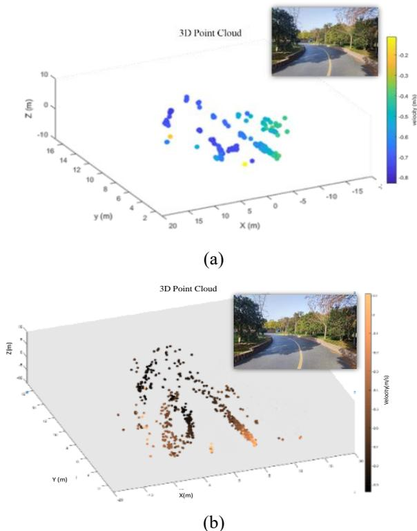
Fig. 15. The roadside imagery using (a) the original method of TI AWR2243 and (b) the proposed method.
