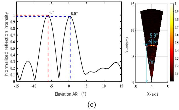
Fig.12. Angular resolutions test with (a) the experiment scenario deployment and the measurements of two targets (b) in azimuth and (c) in elevation.
