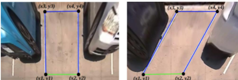
Fig. 4. Polygon parking model for perpendicular and fishbone cases. Entrance lines are marked in green.
