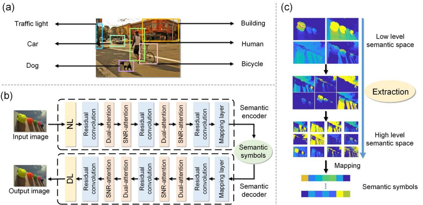
**Fig. 3** (a) Semantics of an image based on human comprehension. (b) Overview of the designed DR-net. (c) Image semantics flow. NL: normalization layer; DL: denormalization layer; Res-block: residual convolution block.
