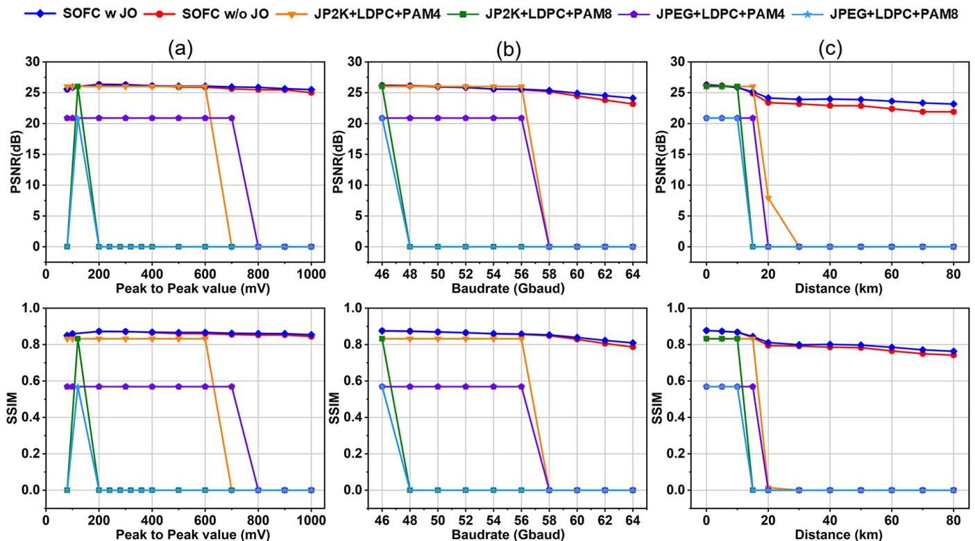
Fig. 5 Transmission performance with respect to (a) peak-to-peak value, (b) baud rate, and (c) transmission distance.
