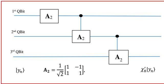
Fig. 6. The quantum circuit for the 3-qubit QPT.
