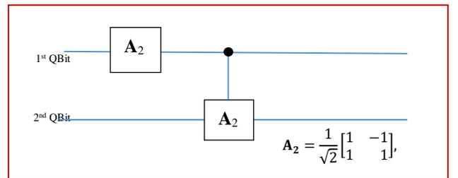
Fig. 2. The quantum circuit for the 2-qubit QPT.
