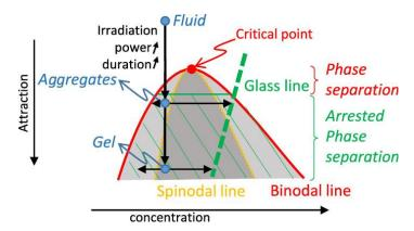
**Scheme 3.** Schematic state diagram illustrating the physical pathway leading to aggregation and gelation. Reprinted with permission from *J. Phys. Chem. B*, **125**, 12063–12071 (2021). Copyright 2021 American Chemical Society.
