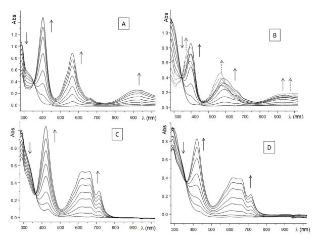
**Figure 2.** Superposition of UV/Vis spectra recorded during the exhaustive reduction (one electron per viologen subunit) of A) **1**, B) **2**, C) **7** and D) **8** (4  $10^{-4}$  mol L<sup>-1</sup> in viologen subunits, DMF + TBAP 0.1 M,  $E_{app} = -0.8$  V, l = 1 mm).
