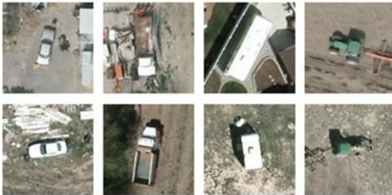
Figure 1. Vehicle Detection in Aerial Imagery (VEDAI) sample data showing different vehicles in different orientations from an overhead visible sensor.
