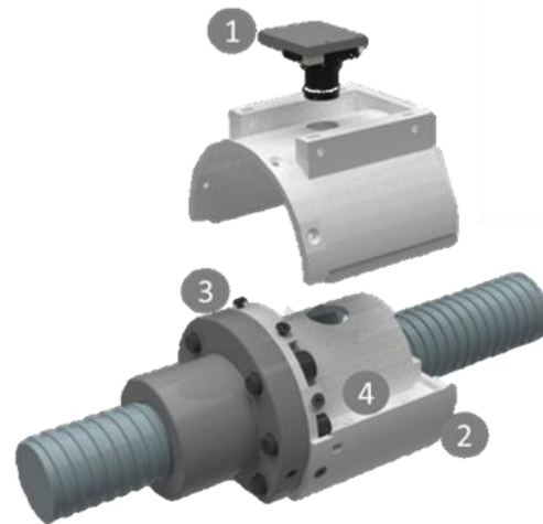
Figure 3: Sensor system used for image generation
