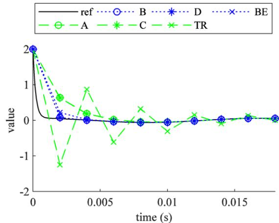
Fig. 11. Transient performance of numerical integrators.
