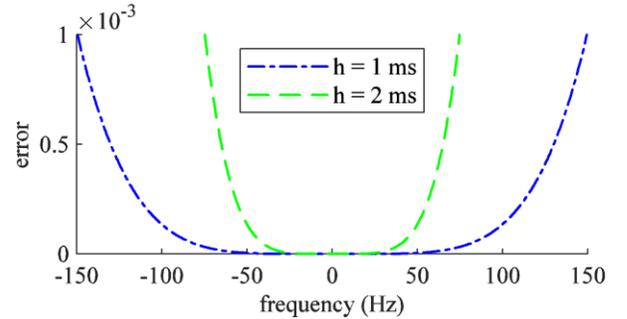
Fig. 3. Magnitude frequency response of the error of Integrator C.
