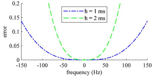
Fig. 4. Magnitude frequency response of the error of Integrator D.
