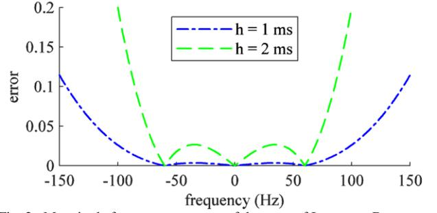
Fig. 2. Magnitude frequency response of the error of Integrator B.
