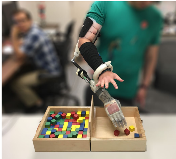
Figure 2. The Box and Block Test provides a quantified evaluation of a prosthetic system. With the bypass socket and DEKA LUKE arm on, participants transferred as many blocks as possible from one partition to another in 1 min. Participants also completed the modified Box and Block Test (not shown), which uses 16 blocks placed in a grid.
