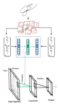
Figure 3 *Top*: Learning features from ATVS dataset. *Bottom*: Convolving and pooling the learned feature for representing the signatures
