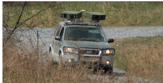
Fig. 1 One of our autonomous vehicles with LADAR sensors on the roof.
