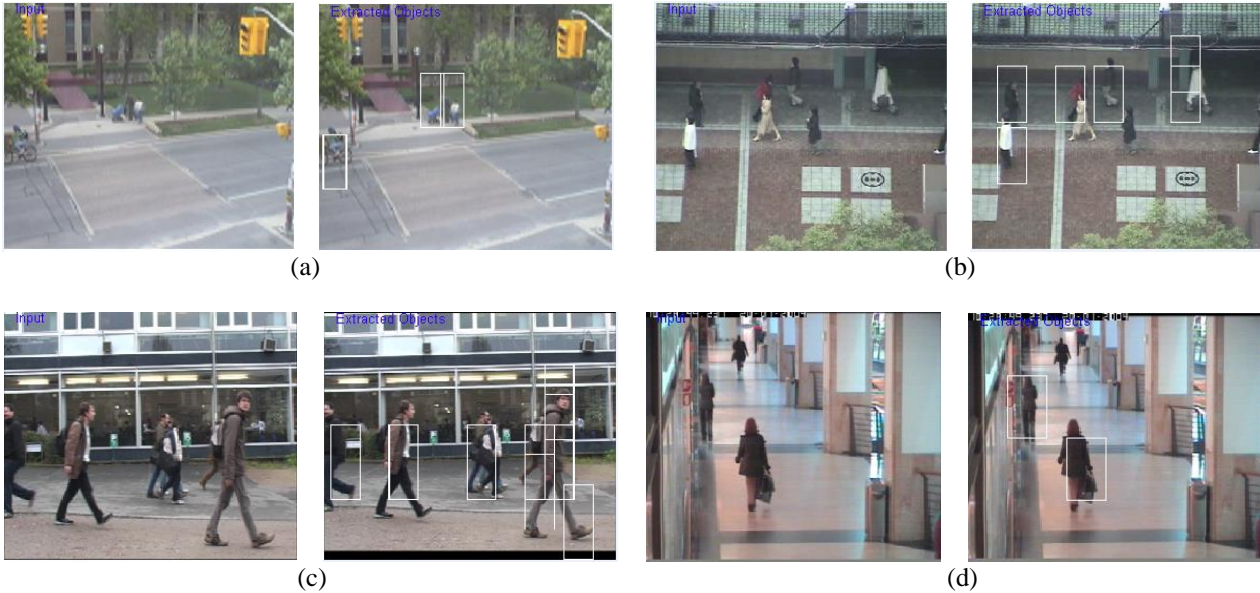
Fig.3. First column indicate inputs and second column is outputs of correspondent input: (a) Road crossing dataset, (b) Subway dataset, (c) TUD campus sequence and (d) Walking dataset.
