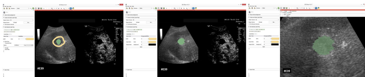
Figure 15. GrowCut segmentation results for a pancreas metastasis. Equivalent to Fig. 14, the left image shows the manual initialization of GrowCut: the pancreas metastasis was initialized with green, and the background was initialized with yellow. The image in the middle shows the segmentation result of GrowCut (green). The right image shows a closer view of the segmentation result (green) with a lower opacity (0.6).
