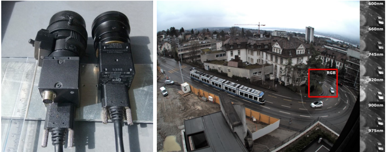
Figure 1. The two cameras fixed on a mounting plate (left) and a sample image of the dataset and cut-outs of 6 from the total of 25 channels of multispectral data (right).
