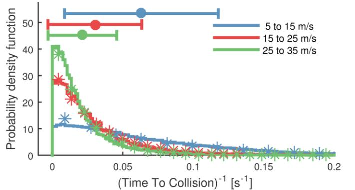
Fig. 8. Distribution of  $TTC_L^{-1}(t_{LC})$  at different lane change vehicle speeds
