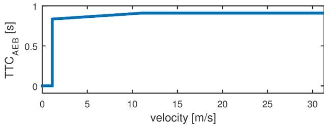
Fig. 12.  $TTC_{AEB}$  as a function of vehicle speed
