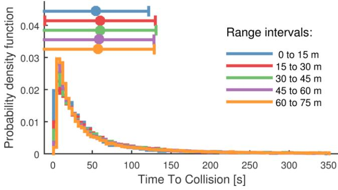
Fig. 10. Distribution of  $TTC_L(t_{LC})$  at different range intervals
